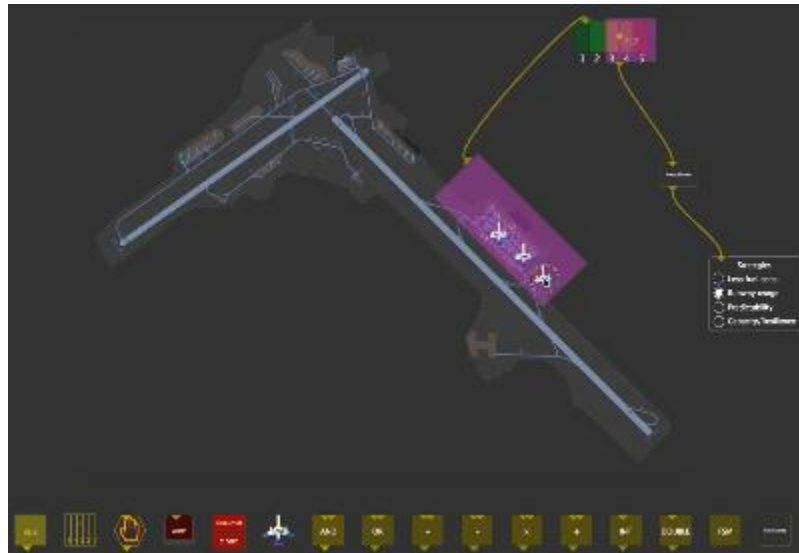
Figure 15 – Programming an automatic change of global strategy with the DSGL according to the number of flights at apron 9
